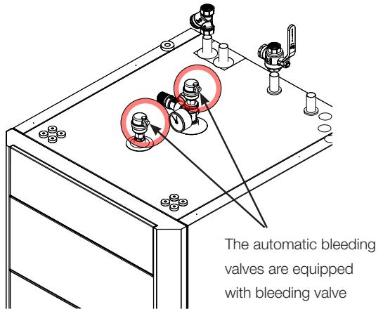
The automatic bleeding valves are equipped with bleeding valve screws.
